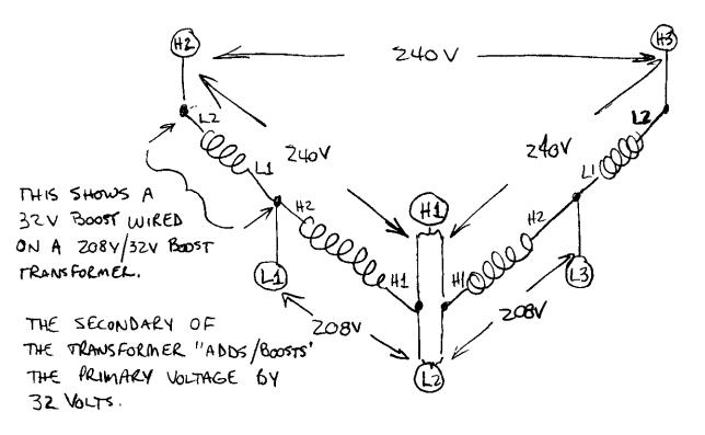
THE RATING OF THE TRANSFORMER IS CALCULATED BY TAKING THE "BOOST" VOLTAGE (I.E. 32V) AND MULTIPLYING BY THE CURLENT OF THE LOAD, PLUS A SAFETY FACTOR.
